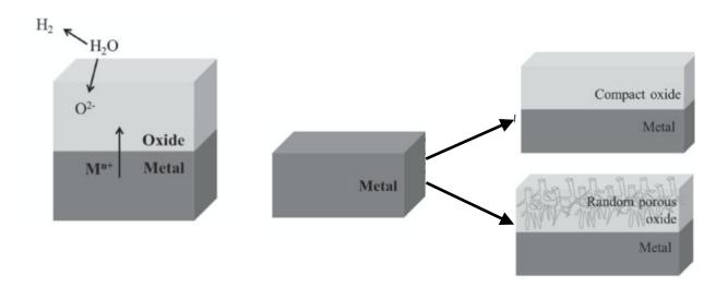
On the other hand, mats like Al forms oxide, whose volume is is greater than the volume of metal (Al). Consequently an extremely tightly adhering non porous layer is formed. Due of absence of any pores or cracks in the oxide film, the rate of oxidation rapidly decreases to zero.
