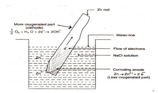
2.2 In a similar way, iron corrodes under the drops of water (or salt solution). Areas covered by droplets, having no access of oxygen become anodic with respect to other areas, which are freely exposed to air.
